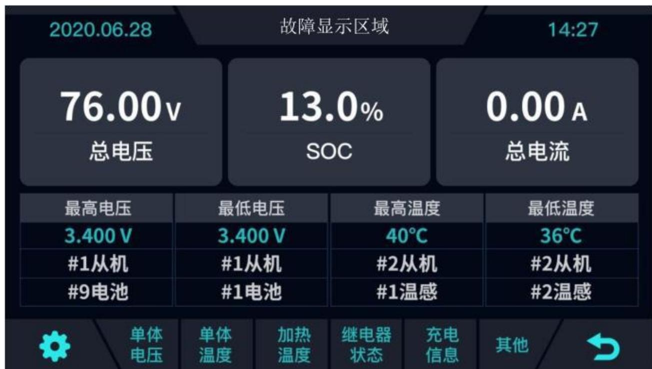
Click on 'Individual Voltage' to enter the voltage details interface, slide left and right to view each string of voltage values, and click
